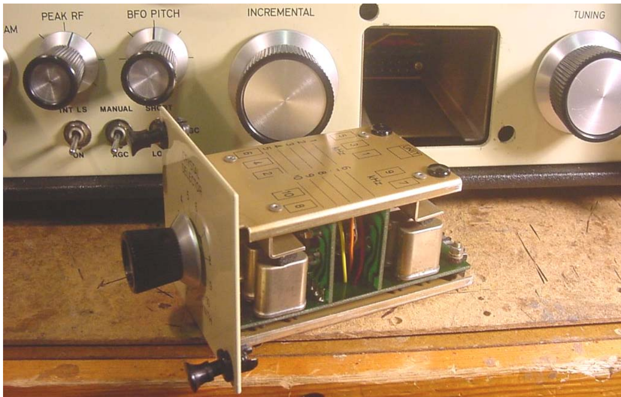
Above: The crystal holder unit removed from the front panel
