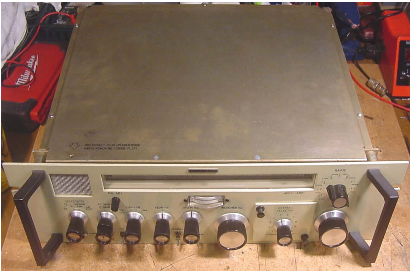
Above: Chassis removed from the outer case, top and bottom covers still in place – this is a very well-screened receiver
